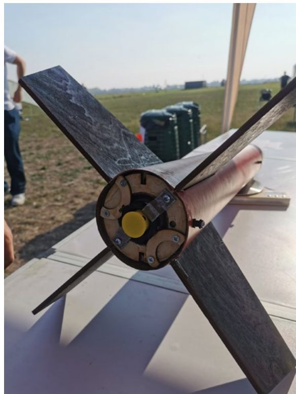
Red Goblin: il razzo sviluppato da Red Propulsion UNIFI DIEF; blocco motore e ugello / Red Goblin: the rocket developed by Red Propulsion UNIFI DIEF; engine mount and nozzle
