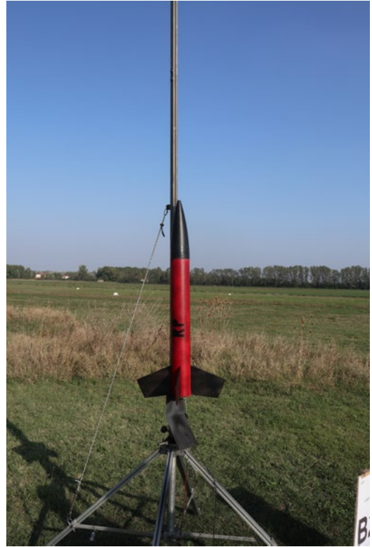
Red Goblin: il razzo sviluppato da Red Propulsion UNIFI DIEF; rampa di lancio / Red Goblin: the rocket developed by Red Propulsion UNIFI DIEF; launch rail
